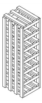
5. Middle Stack and Top Stack rack can be place directly on top.
